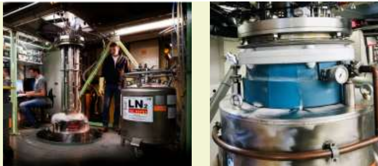
ATLAS, axial +/- 650 kN, RT to 4.2K
