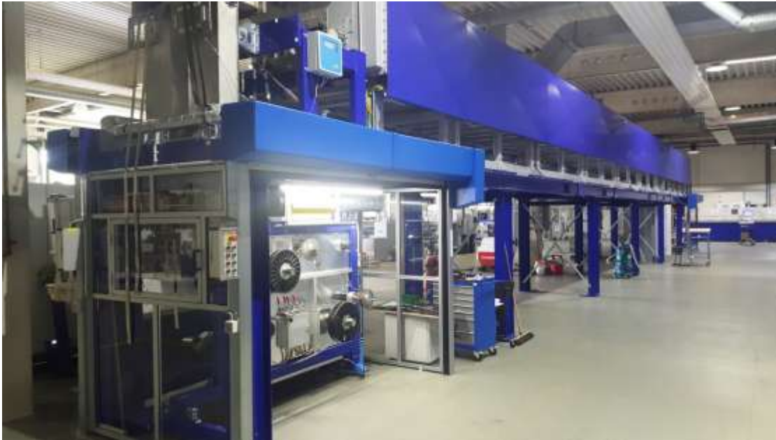
4x25m high temperature annealing furnace
